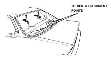
The automatic lap/shoulder restraint system at the front passenger seat cannot be used to secure a child restraint system. Instead, an optional lap belt must be installed specifically for securing a child restraint system. Two anchor points have been provided behind the front passenger seat for installation. The optional lap belt is available from your Honda dealer.
