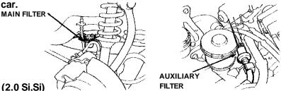
The fuel filter is located in the engine compartment, on the right center of the firewall. It should be replaced at 60,000 miles (96,000 km) or 48 months whichever comes first, or any time you suspect contaminated gas may have clogged it.
