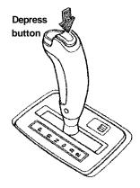
If you cannot shift out of Park with the brake pedal depressed and the ignition switch in the II position:
