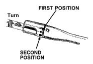
When the switch is returned from the second to the first position, the headlights will go off but will not retract; they retract when the light switch is turned to OFF.
