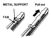
3. Remove the metal retainers from the worn-out blade rubber and put them in a new blade rubber.
