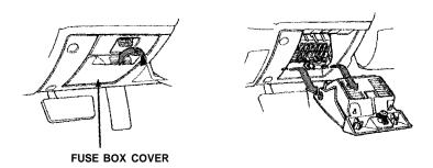
If any of your car's lights, accessories, or controls don't work, check their fuses. If a fuse has blown, the wire inside it win be burned through.
