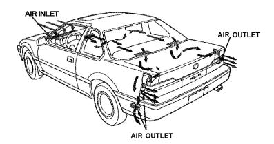
You can adjust the controls to direct cool or warm outside air throughout the car for defogging windows, heating, or cooling by turning on the fan.
