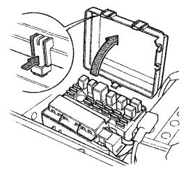
The main fuse and some primary fuses are installed in the fuse box on the right front fender in the engine compartment.
