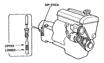
Insert the dipstick and remove it. The fluid level should be between the upper and lower marks.
