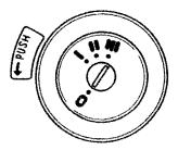
• 0-LOCK position: The key can be removed or inserted in this position. To remove the key, push it in at position I, then turn it to 0 and pull it out. When the key is removed, the steering column will lock.
