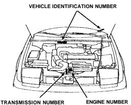
**The Engine Number** is stamped on the right front side of the engine block.
