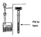
7. Loosen the air bleed bolt in the thermostat housing, then fill the radiator to the filler neck with the coolant mixture. Tighten the bleed bolt as soon as coolant starts to run out in a steady stream without bubbles.
