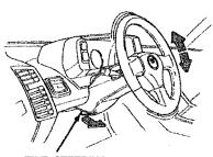
2. To lock the steering wheel, hold it in the desired position and release the lever.
