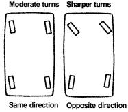
When the steering wheel is turned more than approximately one half turn, the rear wheels are steered in the opposite direction of the front wheels. This reduces the turning radius of the car for easier parking, U-turns, and maneuvering in confined spaces.
