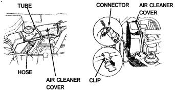
Loosen the wing bolt and unsnap the clips,
