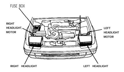
2. Use the label on the fuse box cover to locate the fuse for the headlight motor that doesn't work. Remove the fuse with the fuse remover located in the fuse box under the dashboard.
